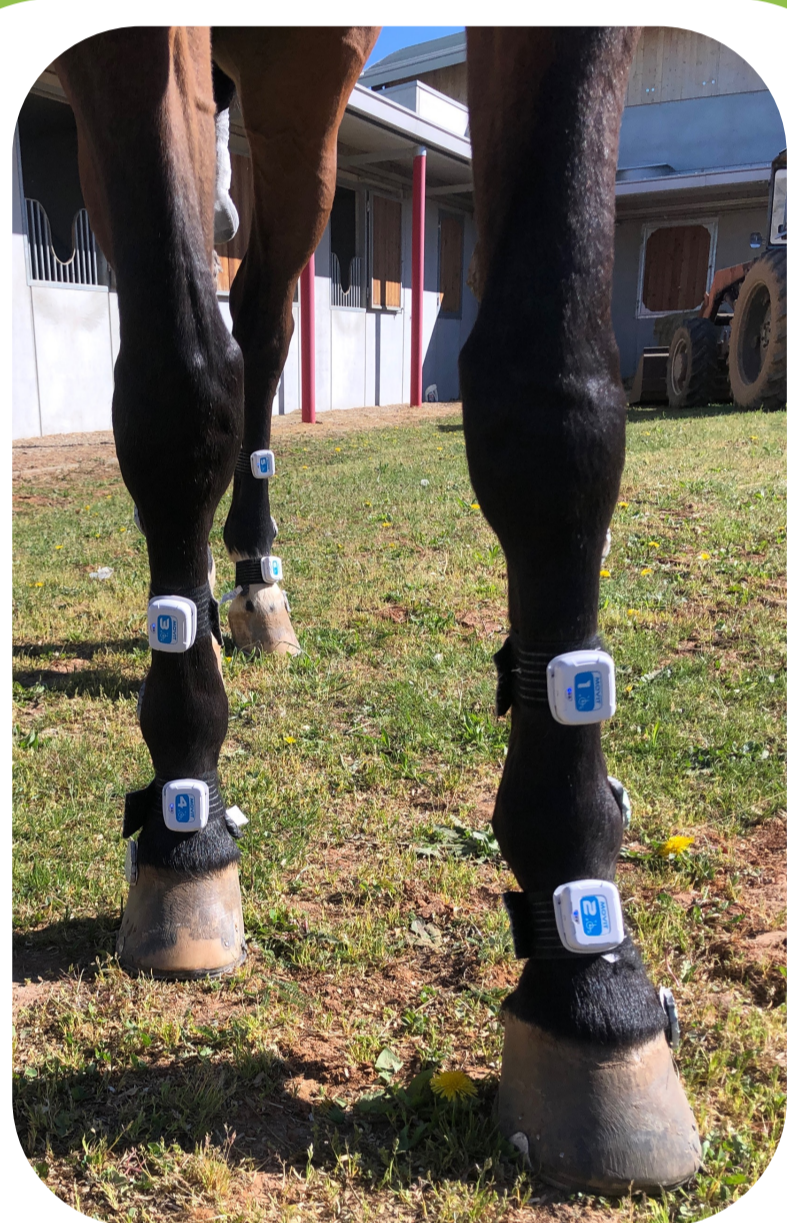
Fig.2 IMUs arrangement without the SS at baseline
